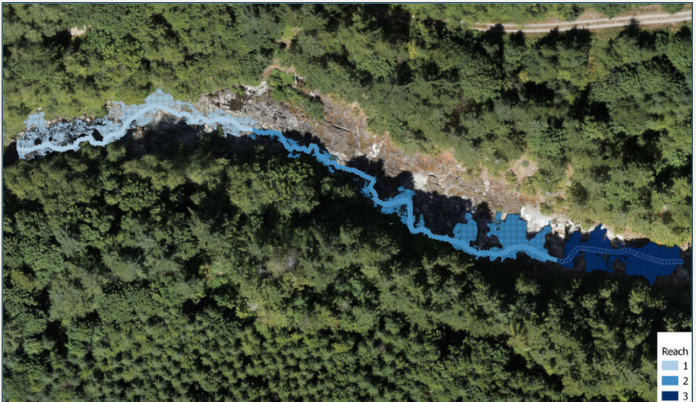
Figure 4: Leech river orthomosaic showing the centreline sample points (circles) and detected wetted area (shaded) for Reach 1 (light blue), Reach 2 (medium blue), Reach 3 (dark blue).
